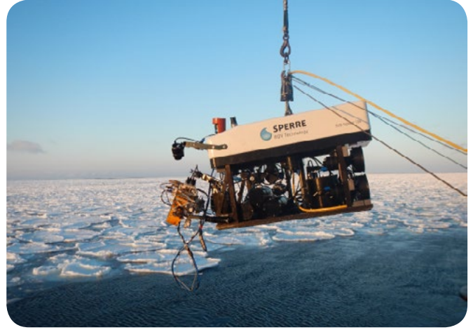
Above shows the ROV with the SpoolScanner on-board being lowered for subsea deployment.
