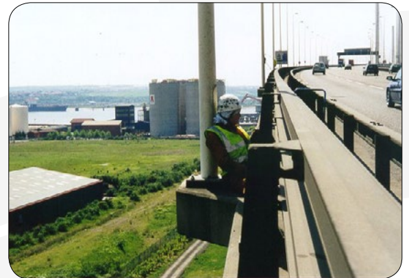
QEII Bridge (cable-stayed bridge opened in 1991) ACFM® inspection of lamp post welds.
