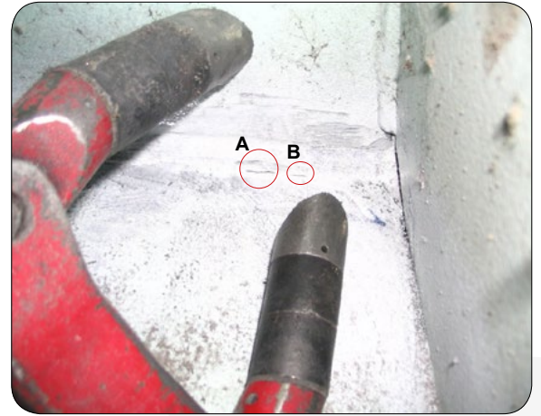
Thames Bridge, built in 1867: ACFM® signals from 2 defects on a bridge weld (left) with MPI indications from the same defects (right). Defect A was 20 mm long by 3.9 mm deep; defect B was 10 mm long by 3.0mm deep.
