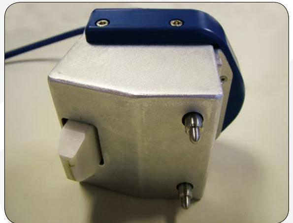
Above & Below: High temperature weld probe with forced air cooling for increased contact times.
