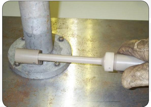
Above: High temperature right angle pencil probe for tight access applications.
