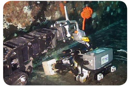
Above shows Meridian's ROV Arm deploying TSC's MagCrawler to the inspection site. (image courtesy of Meridian Ocean Services)
