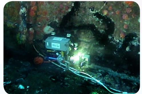
Above shows the MagCrawler working on the Column 4/Pontoon interface "Forward Weld" scan. (image courtesy of Meridian Ocean Services)
